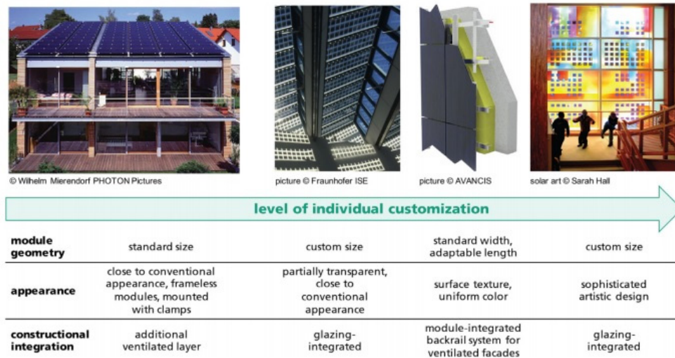
Figure 1: Overview of BIPV systems through examples [2]
