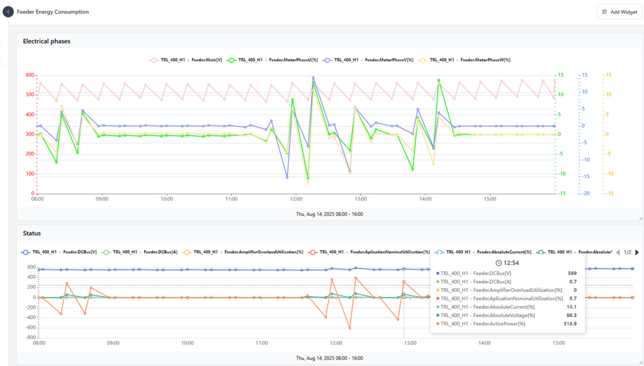
Figure 6: On-line monitoring of energy consumption and electrical health parameters from EtherCAT servo drives for feeder axis [17]
