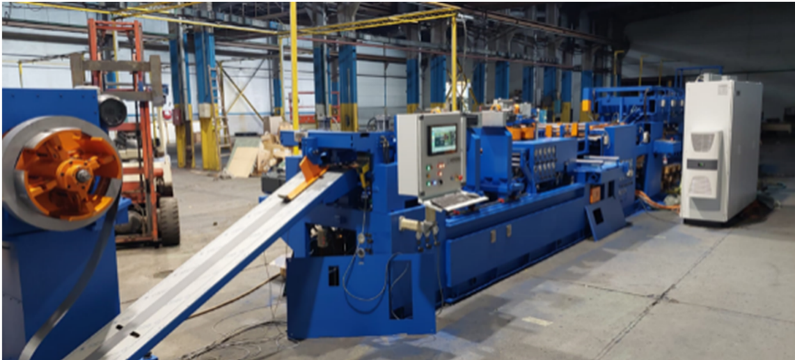
Figure 1: Automated transformer magnetic core cutting line
