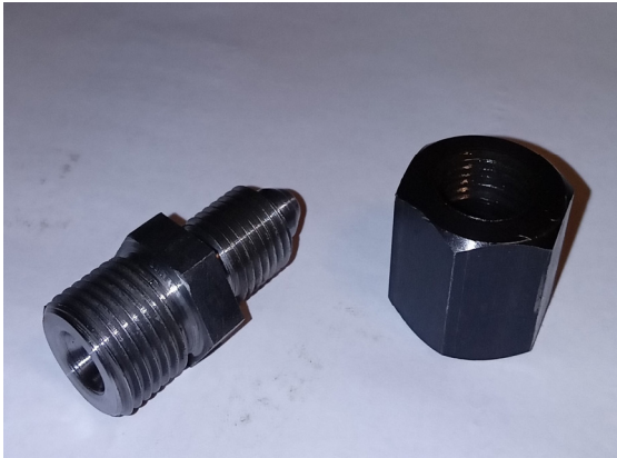
Figure 2: Specially constructed adapters and nuts that have a right-hand thread on one end and a left-hand thread on the other
