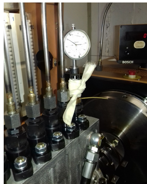
Figure 5: Measurement assembly for determining the pre-lift of the pump element for P500 pumps
