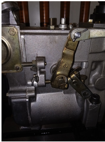
Figure 9: Screws on the body of the all-mode speed regulator on the P10 pump for adjusting the nominal speed and idle speed
