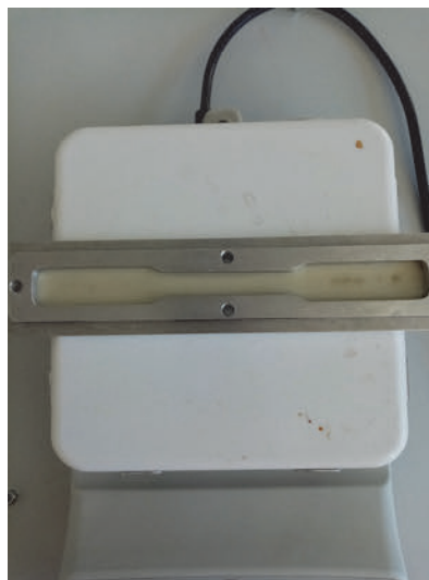
Figure 2: Aluminium mold for the production of tensile test specimens filled with polyurethane-silica sample
