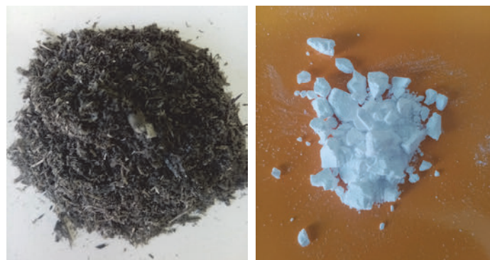
Figure 5: Photographs of samples during the silica powder preparation from wheat straw ash: wheat straw ash (left); extracted silica powder (right)
