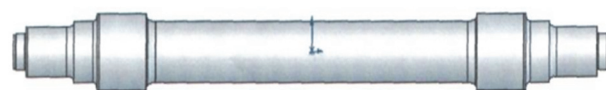
Figure 14: Drawing of the OR 1-1 axis obtained by cutting the ends of an OR 1 axis
