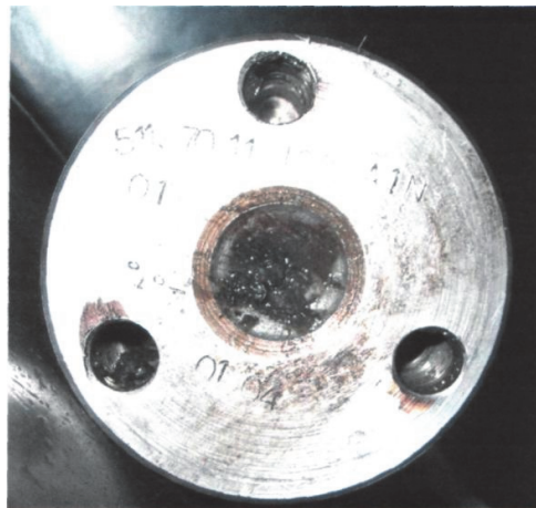
Figure: 10. Traces of heating on the front surface of the broken spindle
